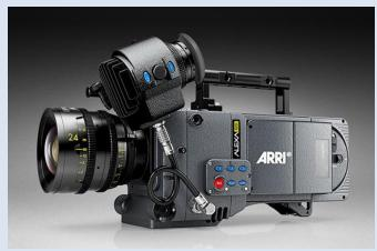
sensor produces images equivalent to that of 65mm film (the so called 70mm film format). In fact the sensor at 54.12 mmm by 25.59 mm is larger than the film gate of a 65mm film camera. Also the sensor has a dynamic range of 14 stops. However, there is a cost to be paid in data requirements; it records at a rate of 2.6 terabytes an hour in ARRIRAW.
