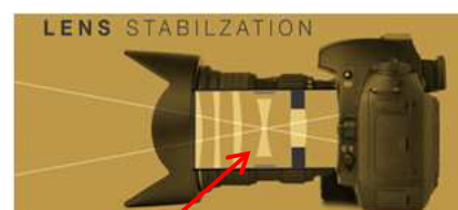
This element “floats” inside the Image Stabilisation Processor
